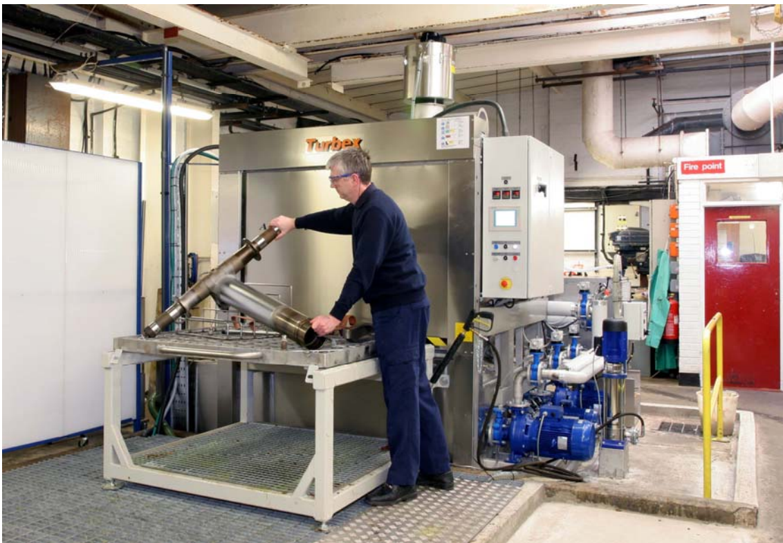
3. The modified Turbex AC-series aqueous washing machine at AEM's Ramsgate centre has just dewaxed and cleaned a Boeing 737 inner cylinder and a jig that held the turning tube for the landing gear of a Tornado.
