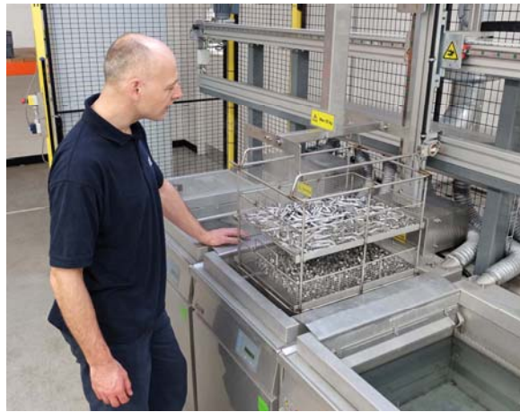
Simon Stowe watching as the carrier is lowered automatically for washing in the second stage.
