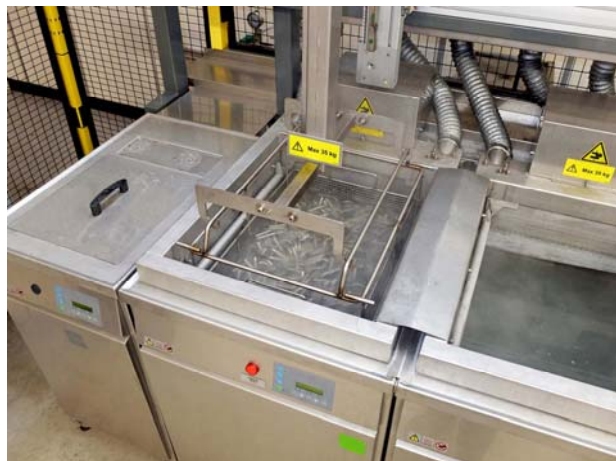
Processing at the first wash stage, with detergent. Turbulation and repeated dunking of the basket carrier assist the cleaning action.
