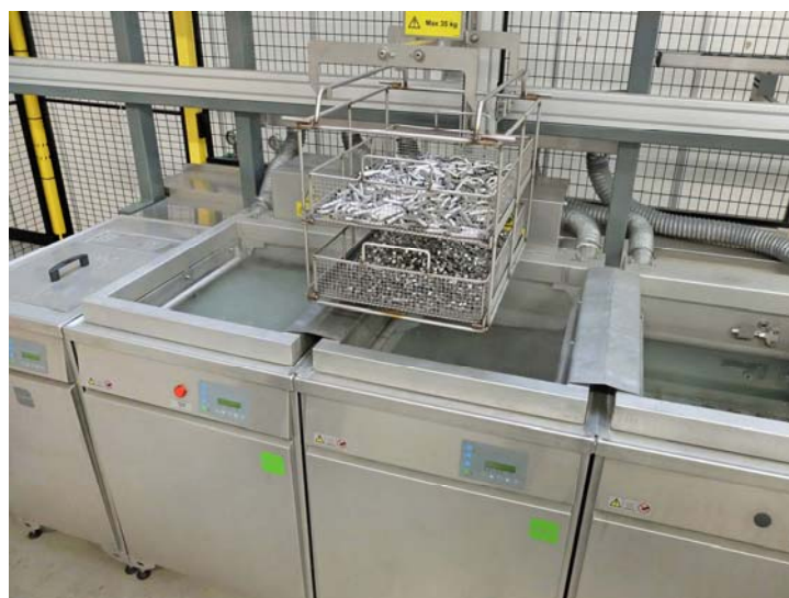
Automatic transfer of the carrier to the second stage.
