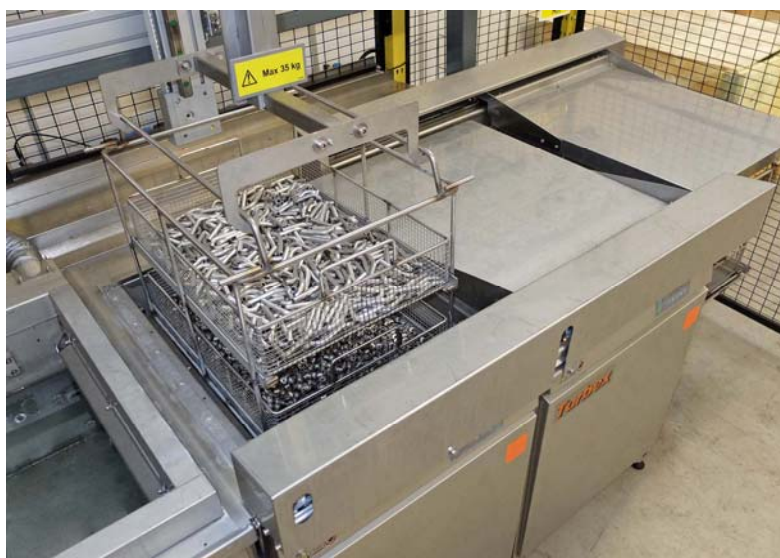
The components about to enter the first of two drying stages.
