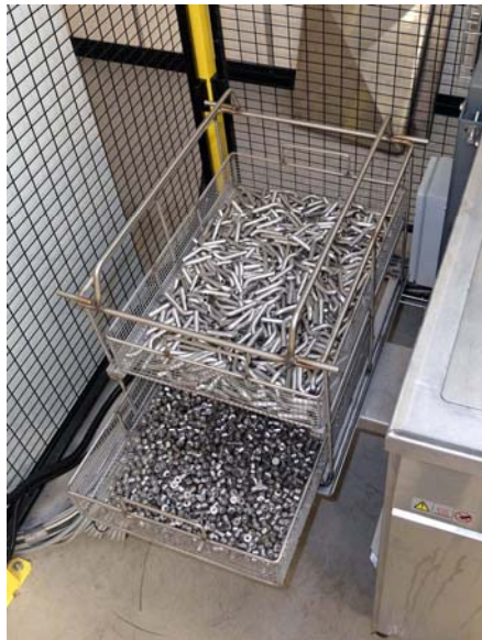
Kanban batches of two different stainless steel fuel rail components ready for cleaning in the Turbex line.
