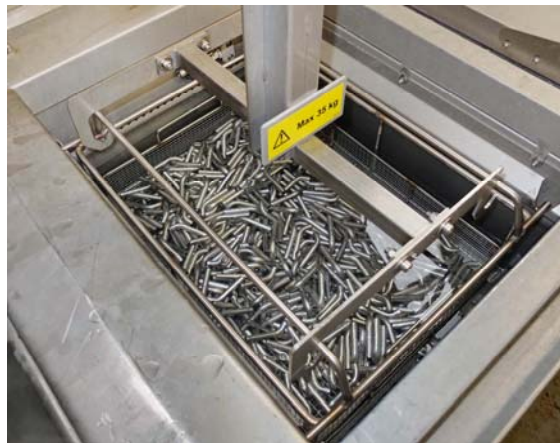
The deionised water rinse tank. By this time, the level of component cleanliness is very high.
