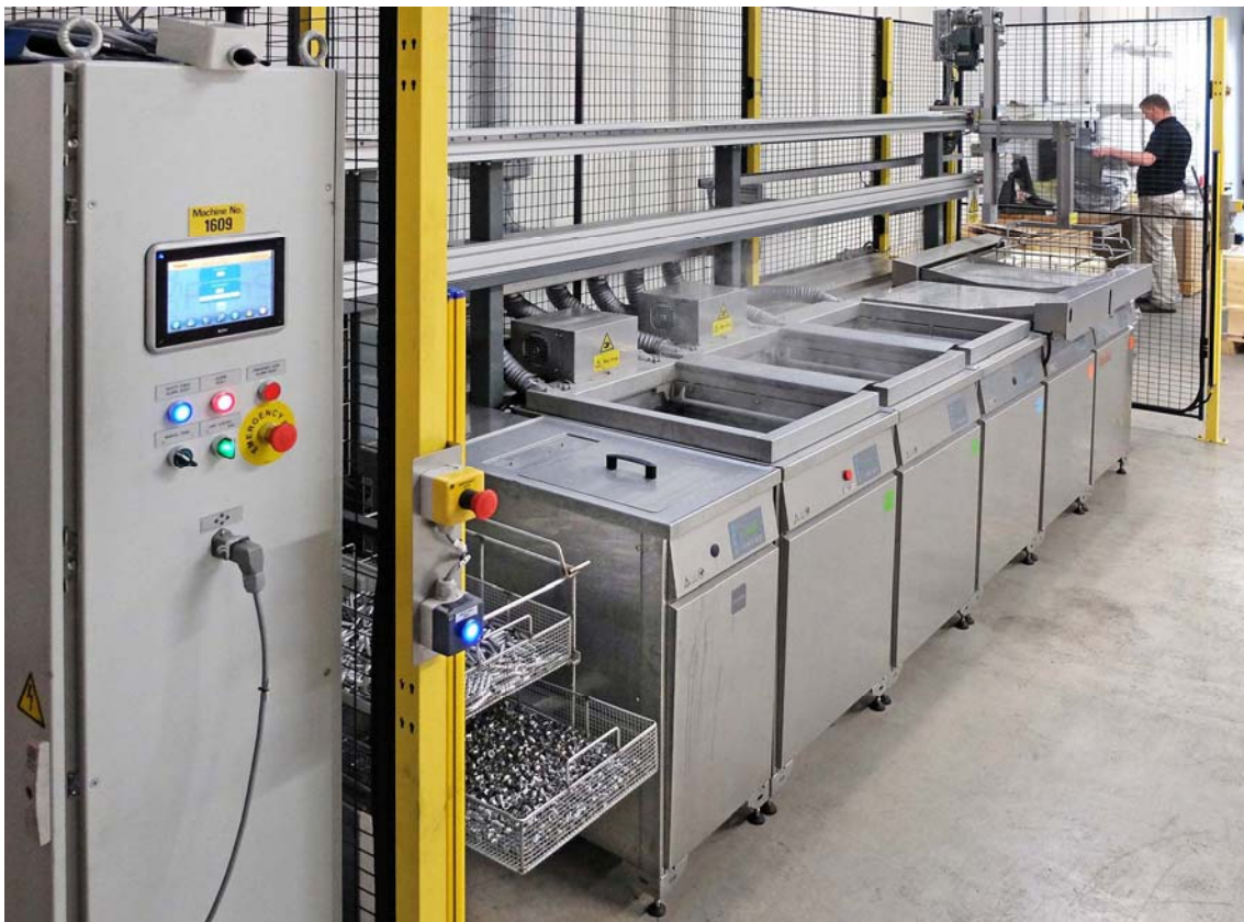
The Turbex automated, five-stage cleaning line at Unipart Powertrain Applications, Coventry.
