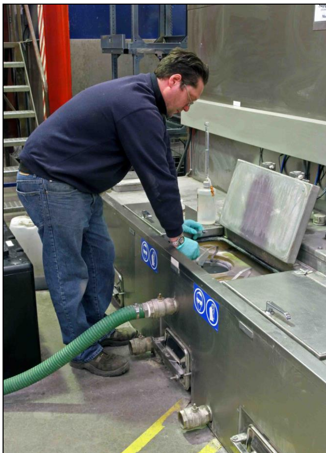
The iron phosphate tank of the Turbex AC-2.5-3 washing machine being checked at Propak.
