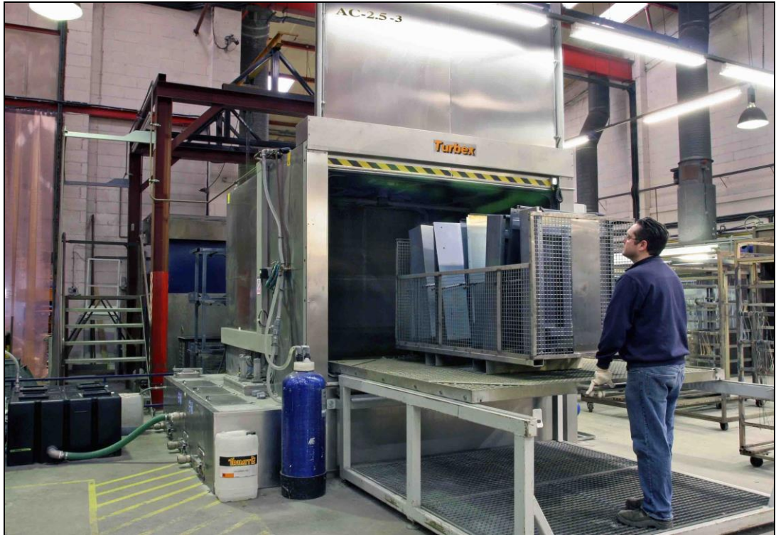
The Turbex AC-2.5-3 aqueous cleaning machine in use at Propak's Stevenage factory. The old trike dip tank that is due for removal may be seen in the background.
