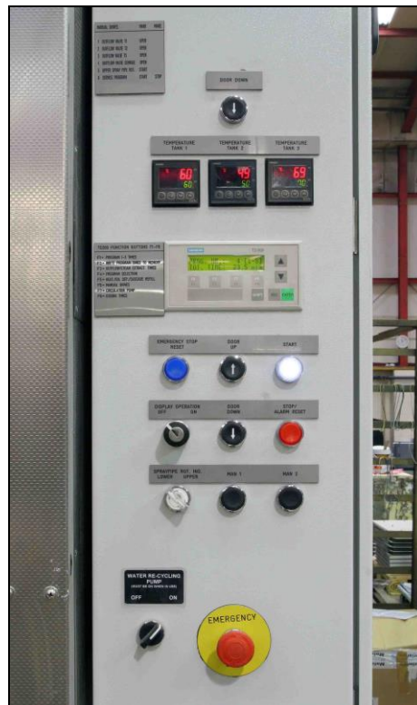
The control system of the Turbex AC-2.5-3. Flexibility of programming and efficient, multi-stage processing elevates industrial component cleaning to a level above that of trike dip tanks, says Propak.
