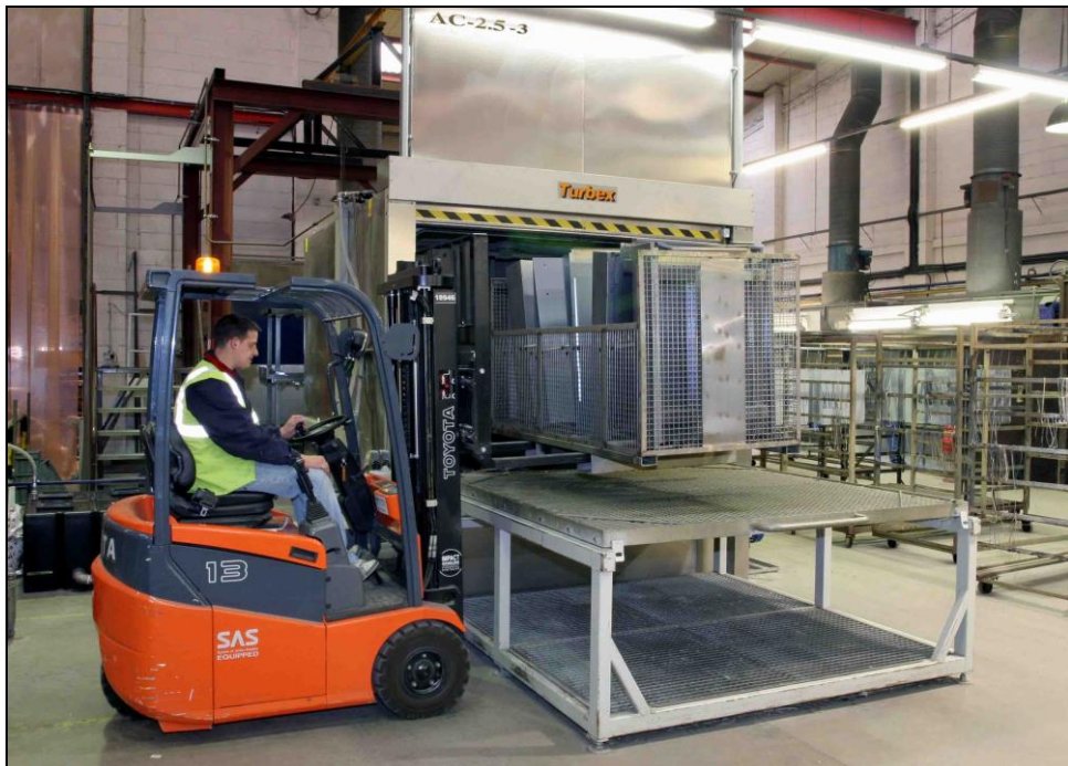
Cleaned sheet metal components being removed from the sliding table of the Turbex AC-2.5-3 at Propak.
