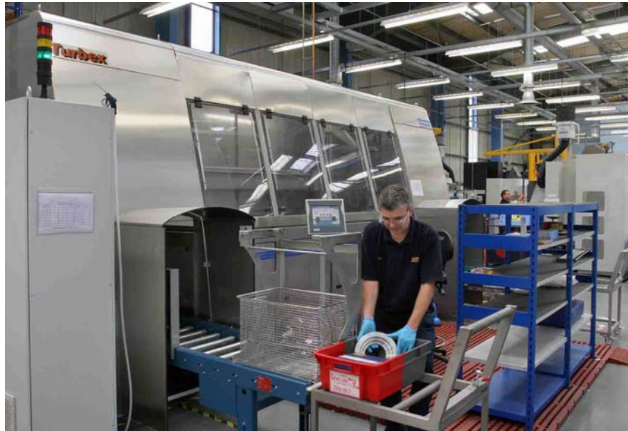
The Turbex / FinnSonic Crystal CRX four-stage washing machine at John Crane UK, Slough.
