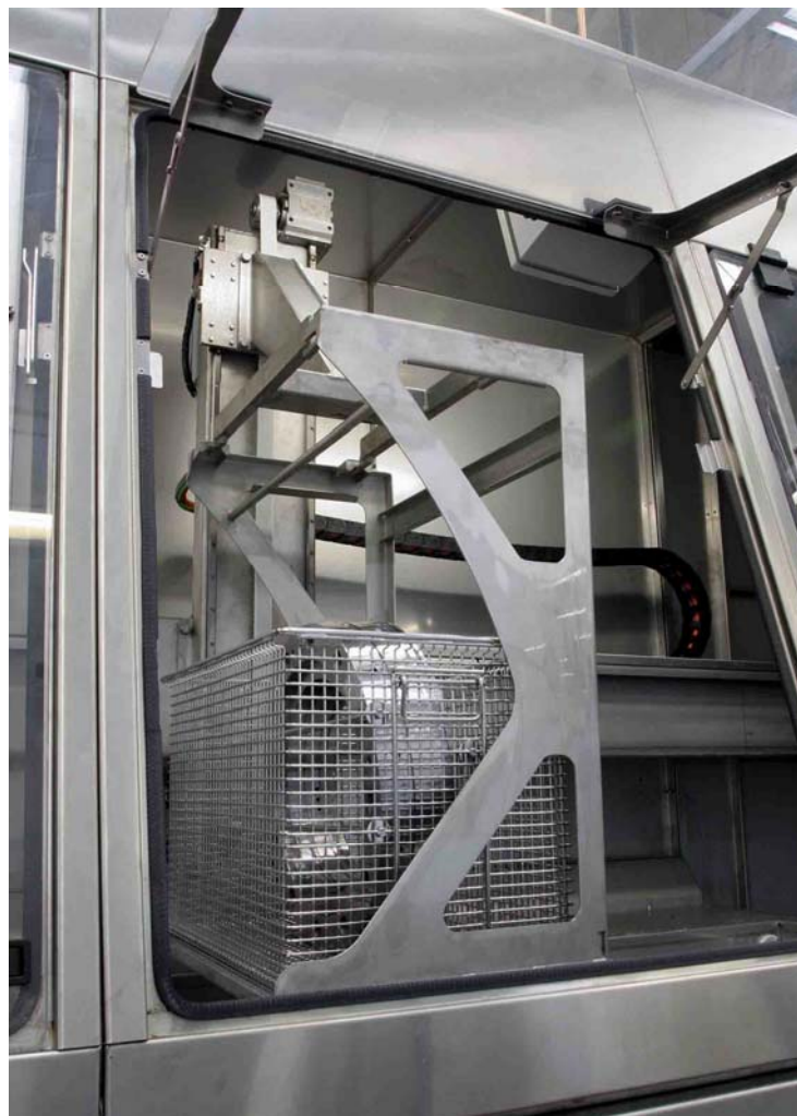
A basket of stainless steel seal components about to enter stage 2 of the Crystal CRX washing machine.
