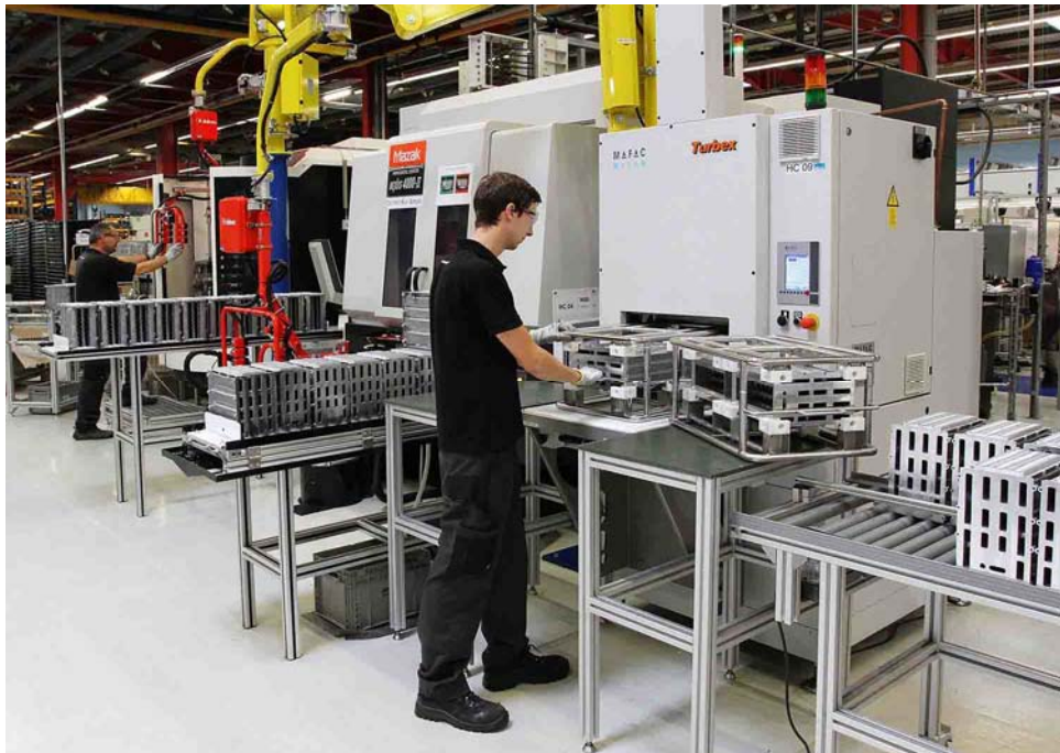
A Mafac KEA aqueous washing machine (foreground) from Turbex in one of the new Worcester heat exchanger production lines. The 4-axis machining centre and friction stir welding machine are pictured centre and left respectively.
