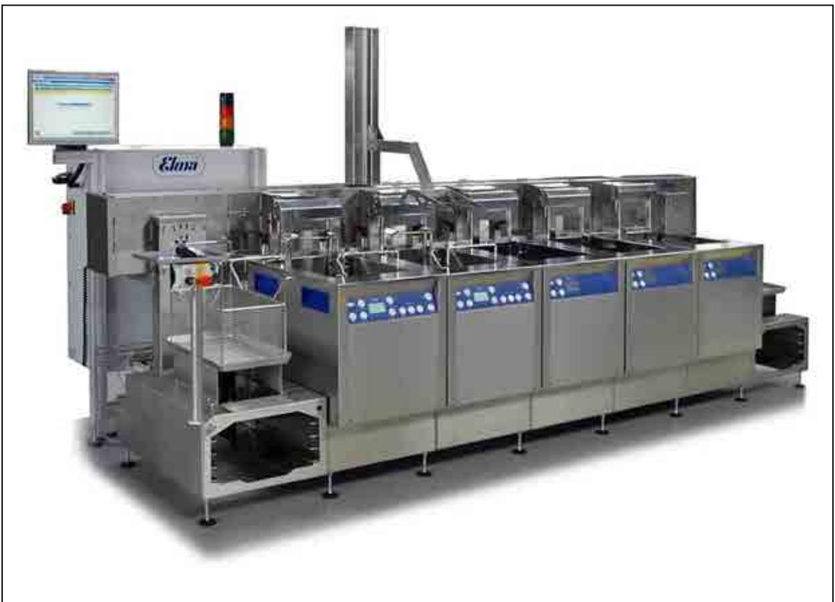
*A high-precision, multi-stage, automated cleaning system from Turbex.*
