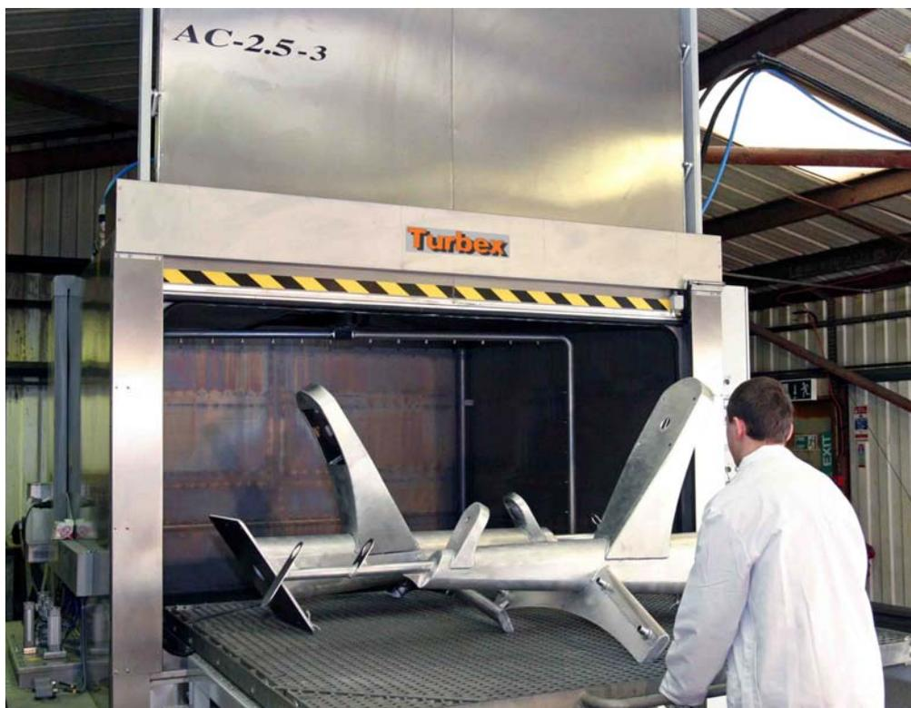
*Radars platforms are some of the larger items processed by Revill in its new Turbex AC-2.5-3-FS-LD aqueous cleaning machine.*
