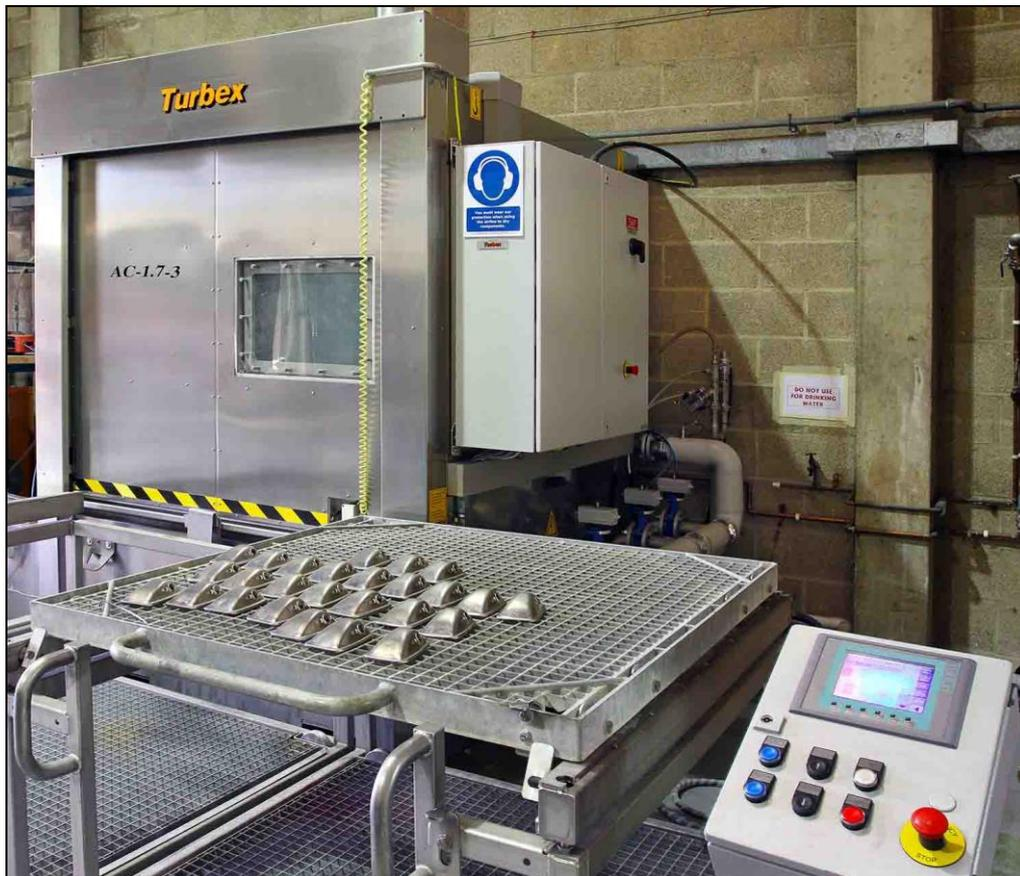
4. While one load is being processed, another is prepared so that it can be immediately loaded into the chamber after the previous load has been removed.
