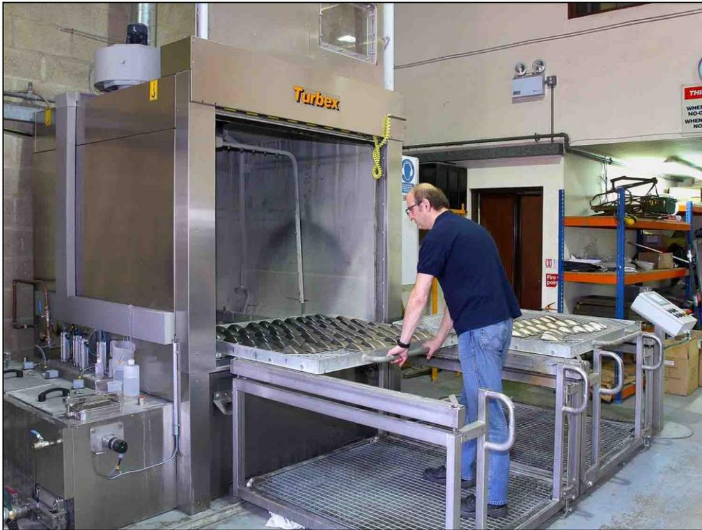
3. One table loaded with wing mirrors being pushed into the Turbex machine.
