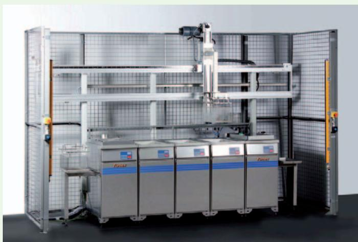
model from its range of spray cleaning machines. Intended for high precision applications, the machine uses a world patented system whereby the movements of the holding basket and the spray jets are individually adjustable,
