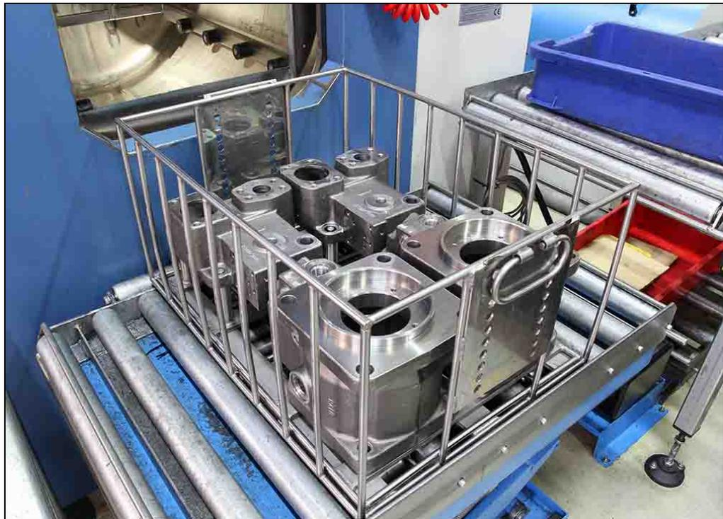
2. A pair of cast iron cases and valve covers for two Kawasaki pumps is clamped into a stainless steel basket, allowing full rotation in the machine while the spray jets contra-rotate.
