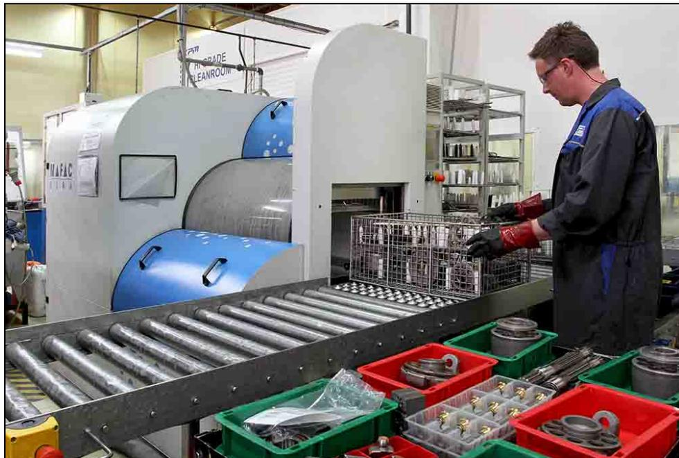
3. Internal parts for a K3VL pump being loaded into a basket for cleaning in one of the Elba machines. They include the cylinder, valve plate and piston, on which the contamination includes lapping paste, plus swash plate and support, shoe plate, servo piston and shaft.
