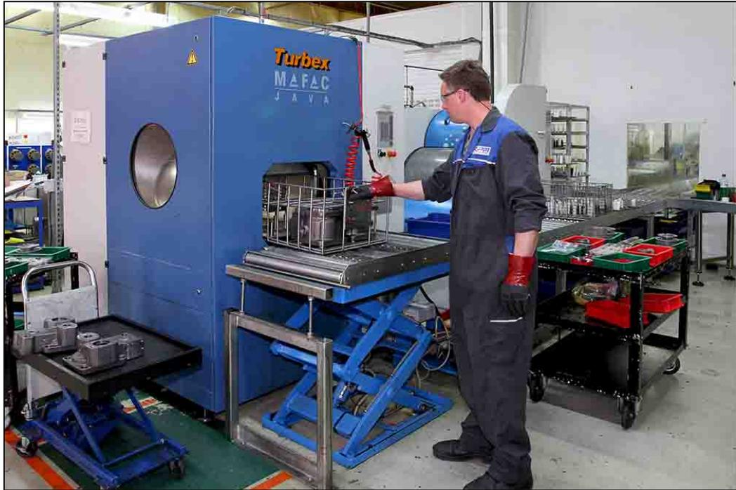
1. The Java being loaded with pump castings prior to cleaning. The Elba that washes the internal parts can be seen behind it. Both machines feed the K3VL pump assembly line through the rear wall.
