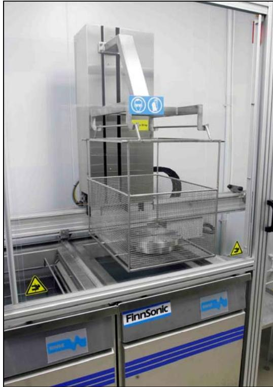
*The basket about to be transferred to the third tank for final ultrasonic rinsing in deionised water.*
