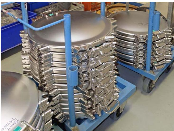
Stainless steel manlids are also cleaned in the Turbex machine prior to fabrication.
