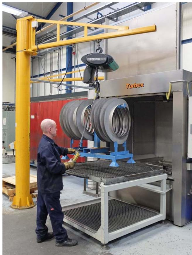
The neckrings being lifted off the table of the Turbex machine.
