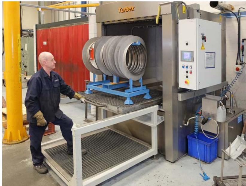
Clean stainless steel neckrings emerging from the Turbex AC-series industrial cleaning machine at Fort Vale's Simonstone factory.
