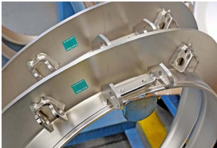
Brackets, which have also been cleaned, welded to the neckrings.
