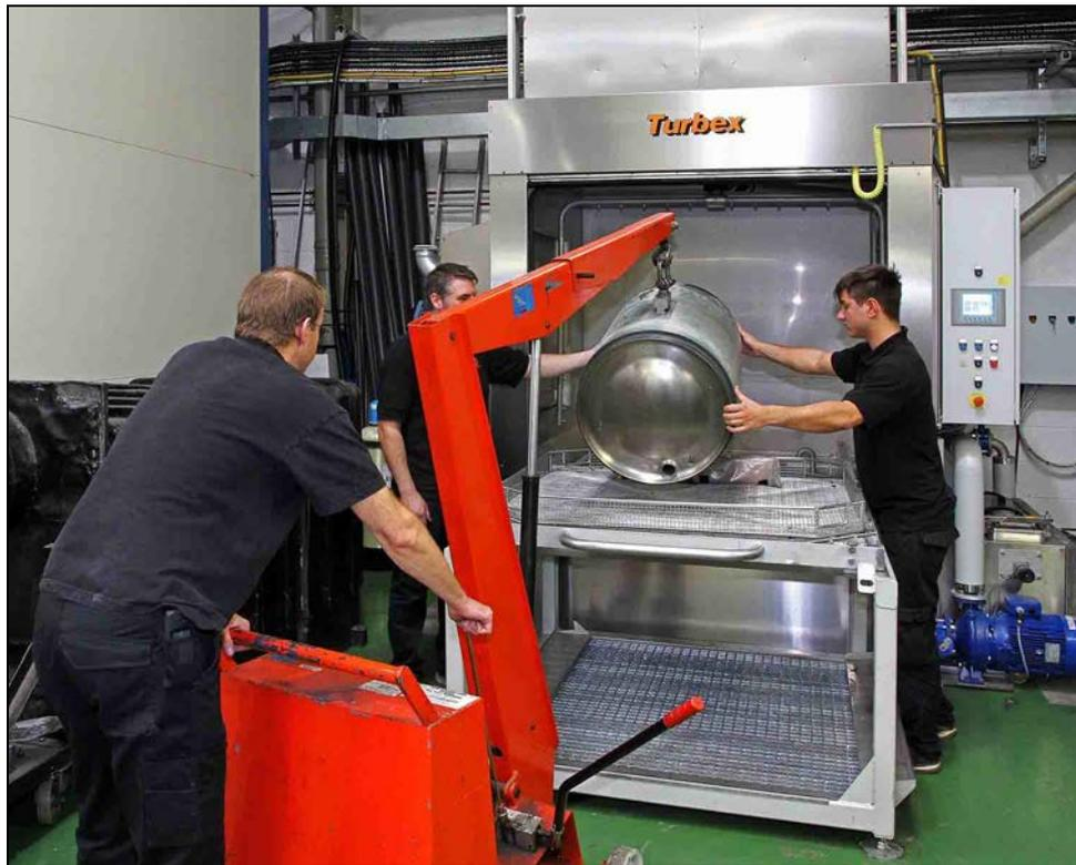
*A titanium fuel tank for a torpedo being loaded into the Turbex at EBP for cleaning.*
