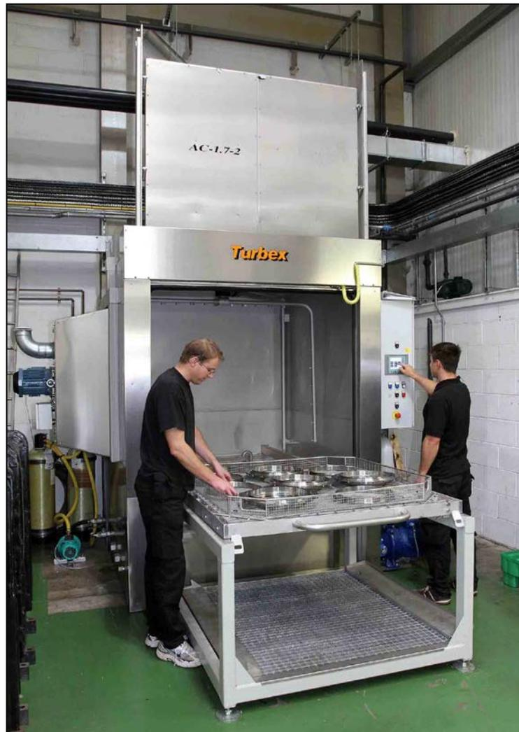
*The Turbex AC 1.7-2 aqueous spray wash machine processing electron beam welded, high pressure bearing housings for the Trent 1000 engine at EBP, Woking.*
