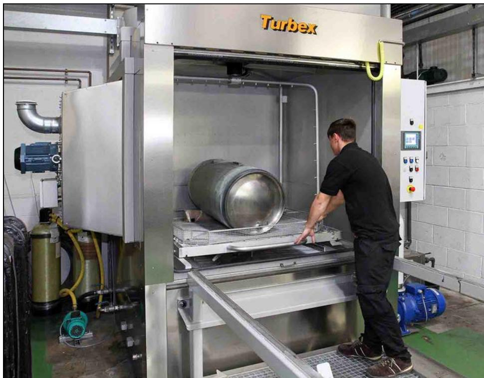
*The fuel tank is pushed into the work chamber.*
