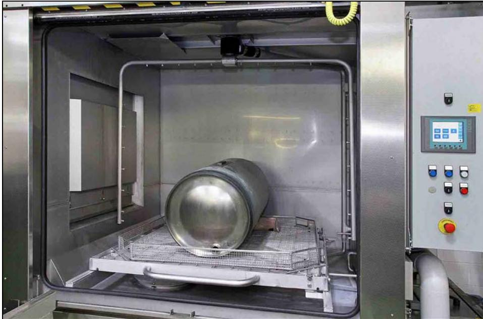
*A view of the interior of the Turbex, showing the rotating spray bars that direct jets of high pressure water onto components.*
