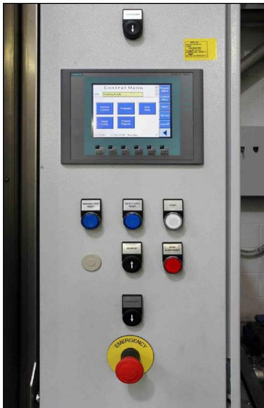
*Almost any wash-rinse-dry cycle can be programmed into the Turbex control system, although EBP uses one proven program most of the time.*
