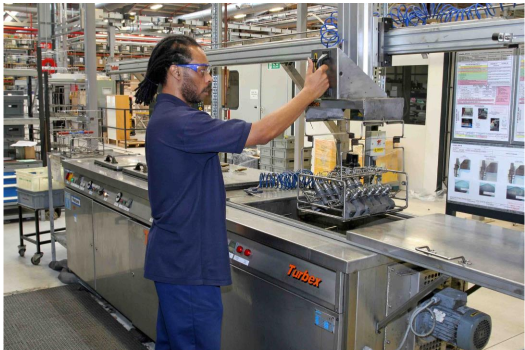
A FinnSonic multi-stage, manually operated, aqueous machine cleaning small quantities of a different design of diesel injector at Delphi Diesel, Stonehouse.
