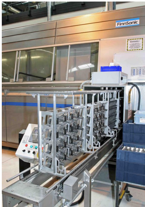
Matched pairs of EUP plungers and bodies ready to enter the A&T cleaning line at Delphi Diesel.
