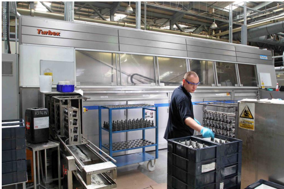
An operator stacking matched pairs of EUI plungers and bodies onto a bespoke wash frame ready for cleaning in one of the BH cleaning lines at Delphi Diesel.
