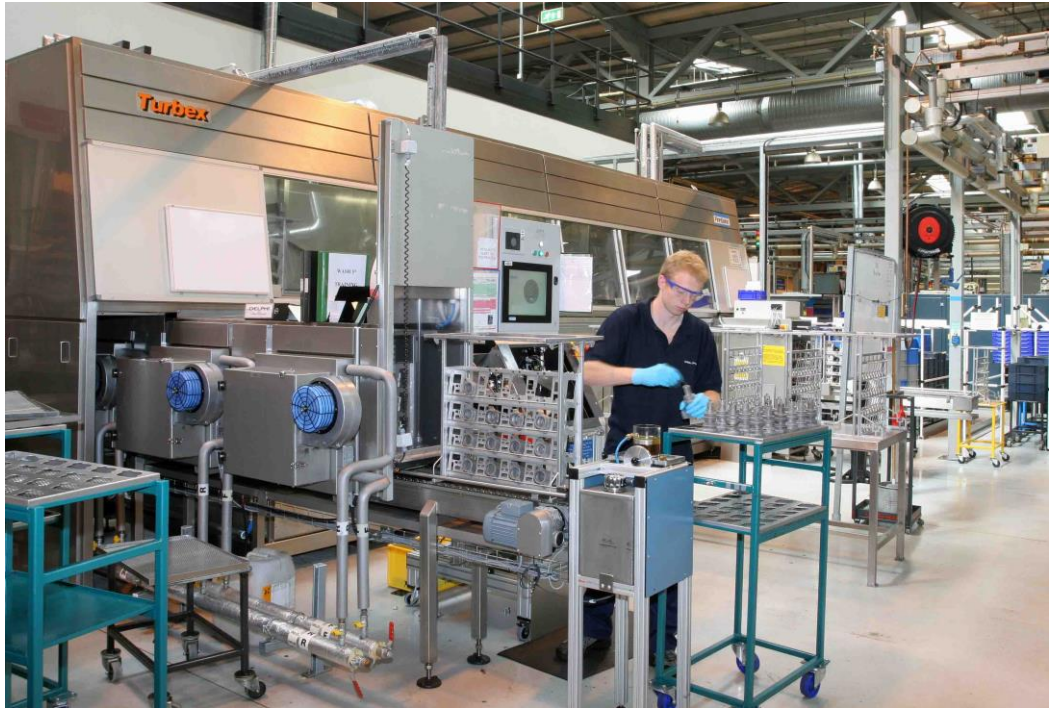
Having emerged from the A&T cleaning line, an operator checks the EUP plungers and bodies, lubricates the plunger and assembles the matched pair ready for injector manufacture.
