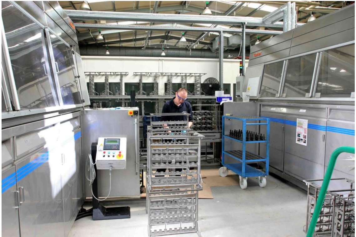
The two FinnSonic cleaning lines in the BH (body hard) area of Delphi Diesel's Stonehouse factory.
