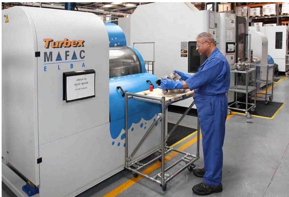
The water pump housing is removed for cleaning in one of two Turbex Mafac Elba machines. The second machine is visible in the background.
