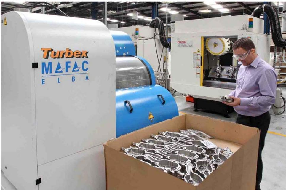
Mark McFall inspecting oil pump housings that have been machined in two Fanuc Robodrills and subsequently cleaned in a Turbex aqueous washing machine.
