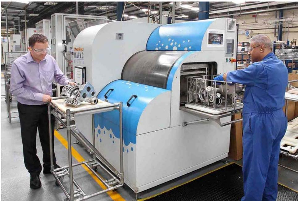
Aluminium pump housings entering the Turbex machine for cleaning. Mark McFall is pictured left inspecting a previously cleaned component.
