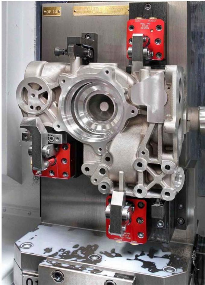
A finish-machined aluminium pump housing in its fixture on a DMG Mori machining centre at Concentric's Erdington factory.
