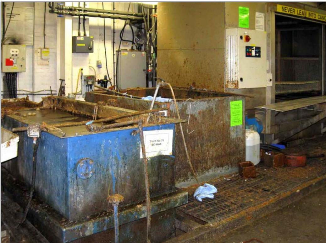
*The previous dewaxing tank (left) and trike tank (right) at AEM, Ramsgate, which would have been used to remove the wax and clean the cylinder.*
