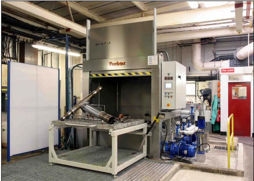
*The modified Turbex AC-series aqueous washing machine that now performs the same job in a single cycle. Dewaxed and cleaned components on the table are the Boeing 737 inner cylinder and a jig that held the turning tube for the landing gear of a Tornado.*
