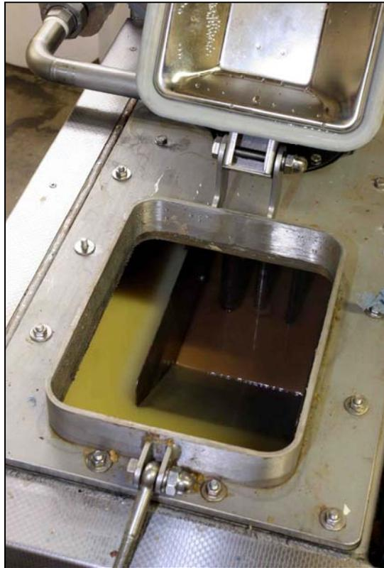
*Close-up of the tank where the oily wax is separated from the top of the water by allowing it to fall into a receptacle and on through tubes, heated by the hot water itself, to the bottom of the unit.*
