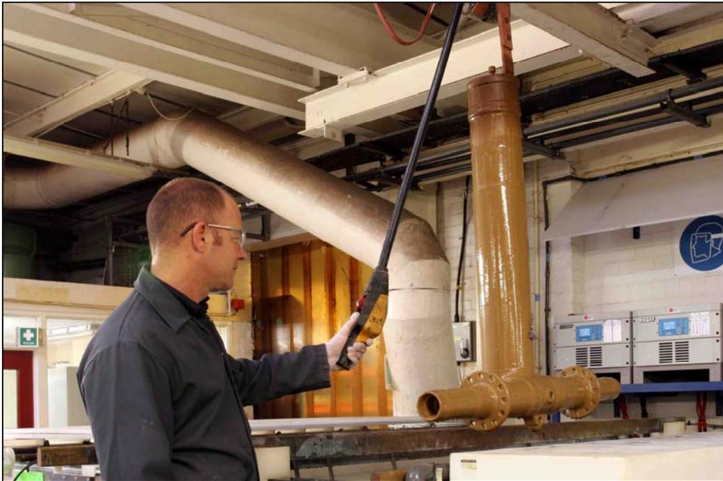
*A wax masked inner cylinder for the landing gear of a Boeing 737 being removed from a nickel plating tank at AEM's Ramsgate facility.*
