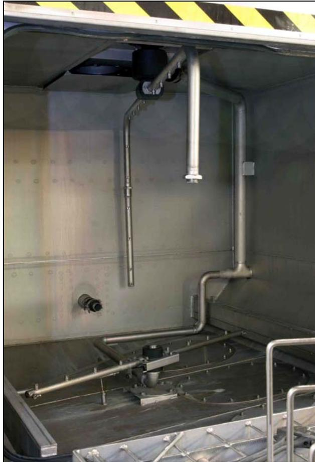
*One of the standard upper spray arms has had the lower section removed so that a small spray nozzle can be fitted. If both arms are shortened, loads approaching the full width of the chamber can be cleaned.*
