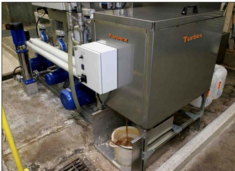
*From there the wax is routed through a separation unit and drops into a bucket below. Water is returned to the system.*
