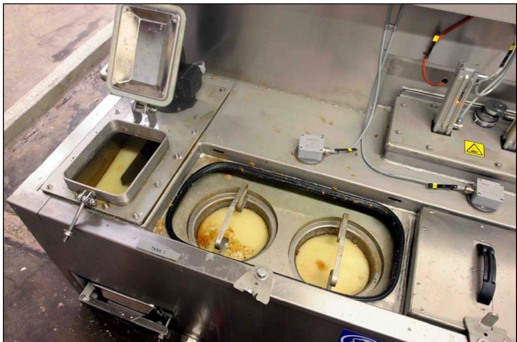
*A view of the wax separation unit fitted to the left side of the Turbex machine.*
