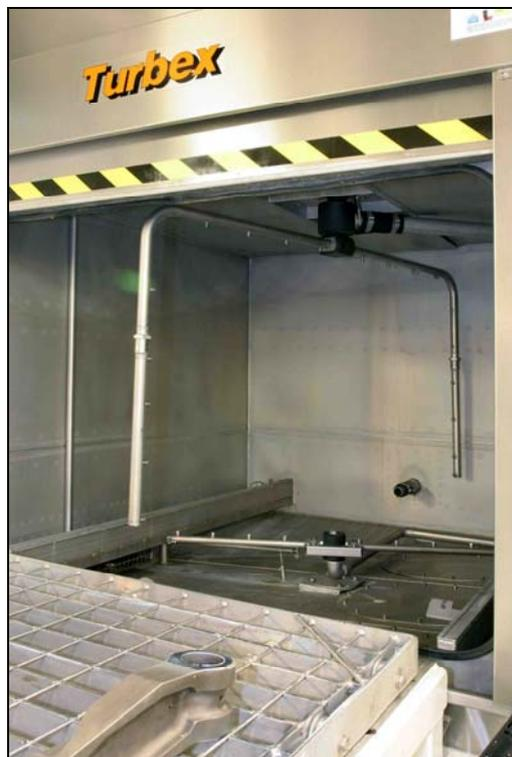
*A view inside the wash chamber, showing the additional manifold for internal de-wax and cleaning installed in the back wall and the modified upper spray arms.*
